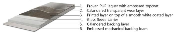
Figure 1: Typical construction
