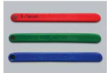
Test objects for metal detectors: plastic strips with a spherical piece of iron embedded in them
