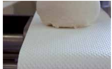
Examples of patterned conveyor belts that can be used in x-ray detectors
