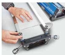
As specified in the Forbo Siegling splicing instructions for different materials, temperature, dwell time and pressure are easy to set. Instructions on the display take the user systematically through the menu. The actual splicing process is carried out automatically.
