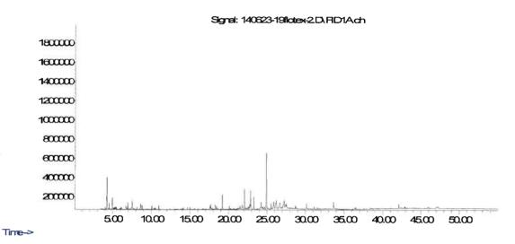
TVOC between  $C_6$  and  $C_{16}$ , means compounds eluting between 5.5 and 36.8 minutes.
