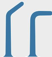
Profiles can be welded to the belts with very narrow tolerances. Nonstandard heights are possible.
