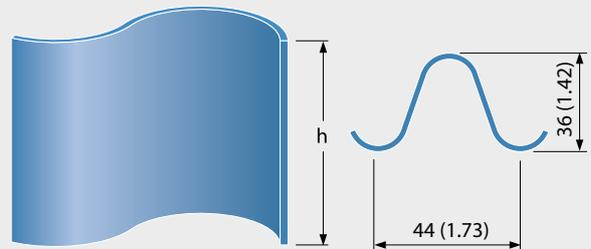
Sidewalls can be welded to the belts with very narrow tolerances. Nonstandard heights are possible.
