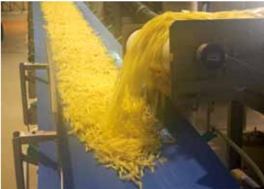
Fullseal is a product family made of homogeneous, thermoplastic polyurethane. All Fullseal belts are completely resistant to oils, fats, moisture and bacteria. They are extremely easy to clean and perfect for use in applications in which hygiene is a priority (e.g. dairy products, dough preparation, meat and poultry processing and other food processing applications).
