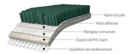
Figure 1: Typical construction
