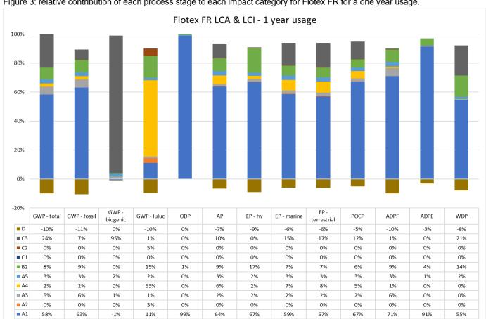
Figure 3: relative contribution of each process stage to each impact category for Flotex FR for a one year usage.
