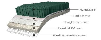
Figure 1: Typical construction
