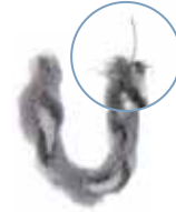
Capillary yarns to absorb moisture and active dirt-scraping yarns
