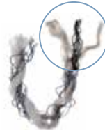
Three yarns: capillary yarns to absorb moisture; active dirt-scraping yarns; and heavy duty texture yarns that can withstand the heaviest traffic.
