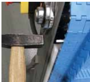
3 Gently tap its head into retaining position
