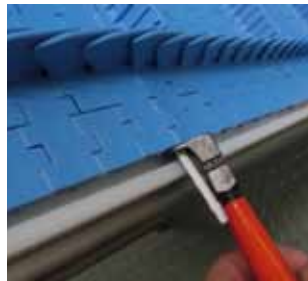
4 Cut protruding rod end slightly behind belt edge
