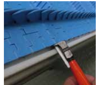
4 Cut protruding rod end slightly behind belt edge
