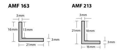
These frames are suitable for smaller matwell dimensions. The bottom foot of the frame is drilled and countersunk so the frame can be secured to the base floor using screws and plugs (not supplied).
