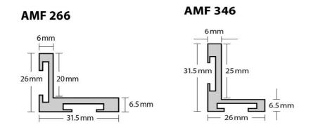
These are clip together frames for ease of installation. They have a formed recess in the frame back and underside to allow insertion of corner and joint plates to hold the frame in place whilst fitting.
