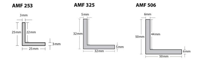
These frames are supplied pre-drilled with corner and joint plates for self-assembly and installation on site. Grouting lugs are also supplied (they anchor the frame into the floor screed for additional strength - see detail below).
