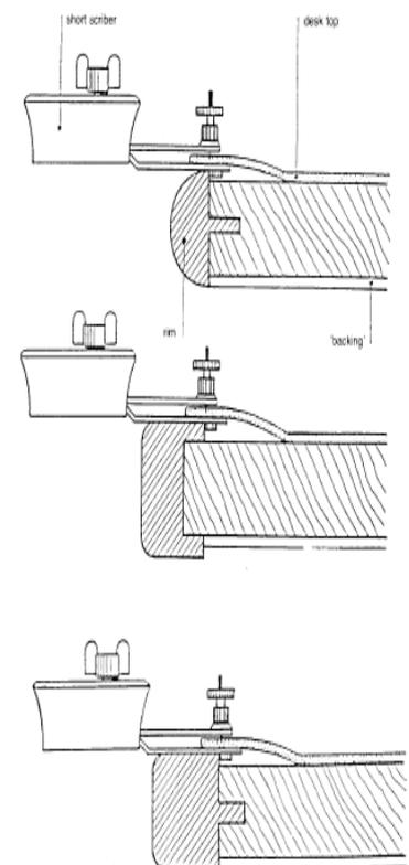
8. Cut the material with a slight undercut along the scribe line, using a hooked blade.
