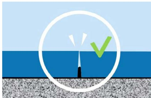
Roll the seam with a seam roller to ensure full contact with the adhesive. Remove any excess adhesive with a damp cloth.
