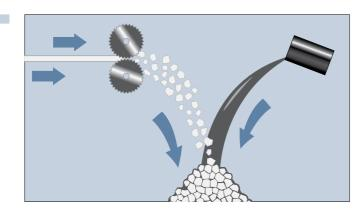
**Step 1: Chips and conductive coating** Small vinyl chips are coated with a conductive substance.
