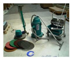
\*) Note: Cleaning/polishing pads for use with single disc machines are usually colour coded according to their degree of abrasiveness. Black is the most abrasive grade, red the least abrasive one. Yellow or white are not abrasive and are used to dry buff the floor for a more shiny appearance.
