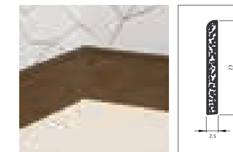
Article reference : PV Ventilated skirtings allow good ventilation of the substrate, especially when an impervious floor is installed (e.g. vinyl flooring, or foil or foam under floorings). After the floor is installed, the profile can be mounted on the wall using screws. A decorative strip covers the screw fixings. Length : 3 m Number per carton box : 20 Colours : 17 or 20 (white)
