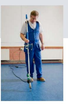
The weld gun holder is attached to the shaft, thus allowing seam welding in an ergonomic position, facilitating work and speed. Hot welding from a standing position is timesaving, compared to the kneeled position. A cable holder ensures a problem free weld cable feed.
