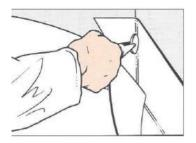
3.1.3 Cut the excess material to the 45-degree angle.
