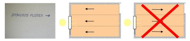
Measure the area to be installed and determine the direction in which the material will be installed and seam placement. Seams must be a minimum of 15cm away from any subfloor joints such as day joints, saw cuts, etc.
