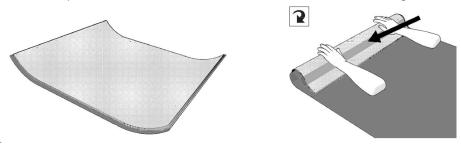
There is an arrow indicating pile direction on the reverse of every backed sheet product. Install sheets with arrows running in the same direction.
