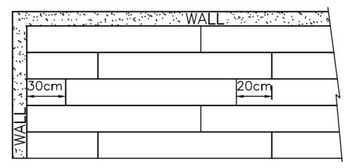
Short 61 x 30.5cm planks: should be installed 'brick' pattern off-set every tile. The offcut from the last panel in a row should be at least 30cm to be used as the first panel of the next row.
