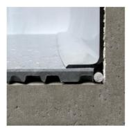
In certain applications, grouting with PUR sealing compound may be reasonable even when skirting are applied.
