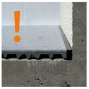
Wrong! A three-sided adhesion of PUR sealing compound inhibits free expansion and may lead to damages!
