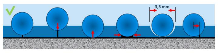
proper depth groove centered Optimum strength weld groove too shallow May "blow out" Weak weld groove too deep Hard to weld Weak weld seam gapped too wide Hard to weld Weak weld seam grooved too wide Hard to weld Weak weld groove not centered Weak weld
