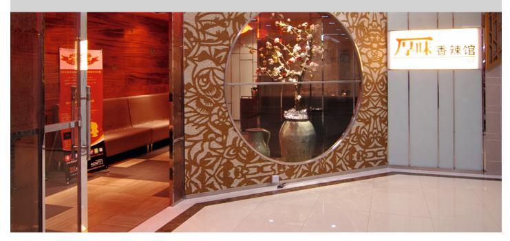
Linoleum is a natural material with attractive design but this time it was used on the walls in combination with a natural stone floor. A digital printing process was used for the pattern which allowed the complex design to be applied most effectively to the linoleum.
