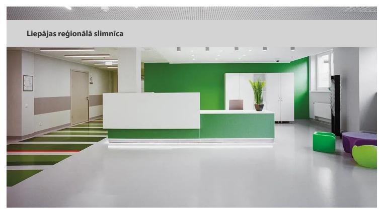
Liepāja Regional Hospital, the largest inpatient and diagnostic center in Kurzeme, Latvia, provides multi-profile emergency and planned medical assistance. Forbo Flooring materials such as Sarlon acoustic vinyl and Sphera Energetic homogeneous vinyl are used in the hospital's interior renovation, with strip patterns in varied colours for the floors of the wards, offices and circulation areas.
