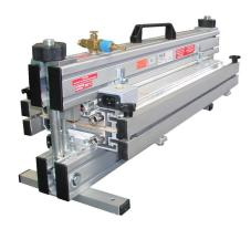
Heating press for melt splices SM-HP-120/300-P
