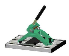
Punching presses of the PP-ZP-V/80-3 type are used for preparing Z-splices for belt widths of up to 80 mm and belt thicknesses of up to 3,2 mm. The splices are 35, 70 and 100 mm long.
