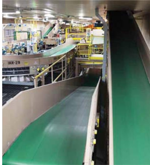
SEW Eurodrive provided gear motors with motor-integrated variable frequency inverters. With this gear-motor/vfd configuration, engineers were able to decrease the number of drive combinations by more than 50%, relates Jan Lindholm, industry account manager at SEW.
