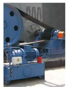
**Kaplan tubular turbines** Turbine power 240 kW Belt type LT 28P
